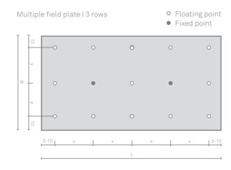
Note regarding horizontal assembly: a grid spacing of max. (y) 600 mm must be observed.
