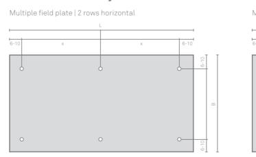
Note regarding horizontal assembly: a grid spacing of max. (y) 600 mm must be observed.
