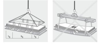
Pallet bending causes cracks or even break of panels. Avoid vibration during manipulation of the pallets. Ensure to load bearing capacity distances. Lift single pallets - do not stack or rest on the edge of the lower pallet. The weight per pallet is usually between 1.5 to max. 2.0 tons. Drive slowly!
