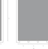
Fixing and edge distances x Wheelbase substructure B Panel width max. 1,200 mm L Panel length max. 3,600 mm
