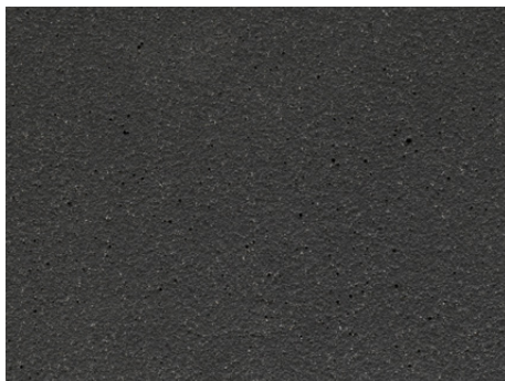
FE ferro sandblasted at high pressure, rough surface
